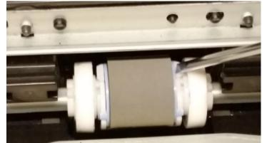
**Step 3:** Clean roller using a clean rag and methylated spirit (or other suitable cleaner) and refit. **Step 4:** Red arrows point to a plastic retaining clip. Push clip together with fingers or other suitable tool.
