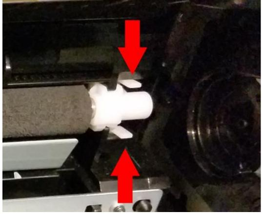
**Step 5:** Clean roller using a soft brush and replace (please note the orientation of the clip).
