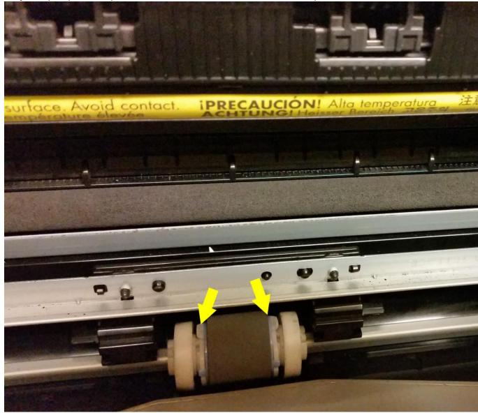
Step 2: Yellow arrows point to plastic retaining clips. Using a screwdriver or other suitable tool - ease retaining clips.
